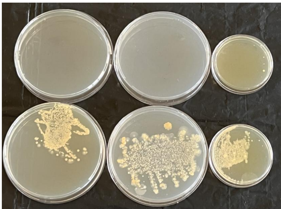
Figure 4. Six plates arranged in two rows. Each row contains three plates representing three types of culture plates: Luria–Bertani (LB), Tryptone Yeast Extract (TYA), and Tryptic Soy (TS). The top row shows plates that were spread with RAS was filtered and no visible bacterial colonies are present on the plate surface. Meanwhile, the bottom row shows non-filtered RAS water, which exhibits bacterial colonies on all three plate types.
